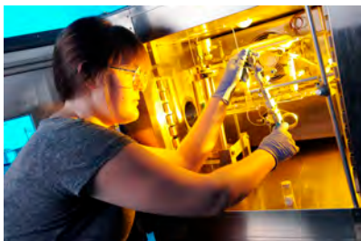
Stephanie Didas, a PhD candidate, prepares a system for measuring adsorption isotherms of different carbon dioxide capture materials
