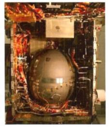
the first four vibration modes of a typical spacecraft cabling segment. At higher frequencies (shear-dominated modes), the models yield modal damping that is either directly or inversely proportional to the mode number. Model predictions compare favorably to available experimental data.
