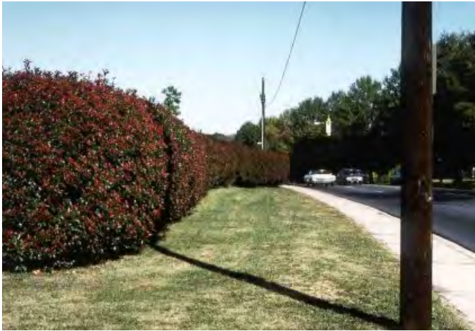
Figure 17: Vegetative buffer Source: www.ncdot.org/doh/preconstruct/pe/OHE/noiseair/barrierpics.html
